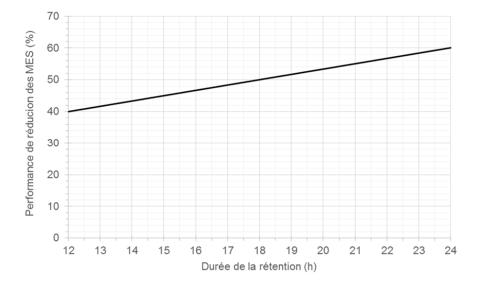
**105.** The dry retention system must have a flow control device for the reduction of suspended matters that ensures a retention period of the runoff volume to be treated of at least 12 hours.
