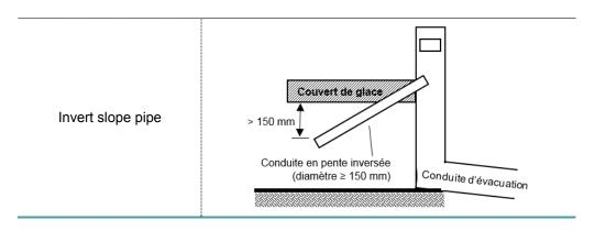
**124.** The end of the protective plate shown in Table 4.4 must be situated at least 150 mm from the ice cover.
