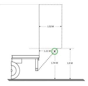
2. With respect to a flexible folding aerodynamic system installed at the rear of a road vehicle, the provisions of the second paragraph of section 4.1 of the Vehicle Load and Size Limits Regulation (chapter C-24.2, r. 31) are suspended and replaced by the following:
